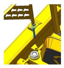
14. Lock the tandem position using the pin provided for this purpose.
