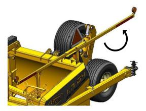
10. Move the tractor to the transport drawbar and connect to it. Use the tractor's hydraulic inlets to lower the drawbar at the tractor drawbar.
