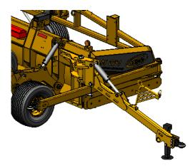
11. Mount the land leveler with the transport wheels and the transport drawbar while maintaining the level of the land leveler.
