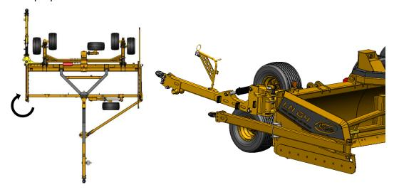
8. Rotate the transport drawbar and lock it in place. Be careful the drawbar must be in the high position to go over the reinforcement arm.
